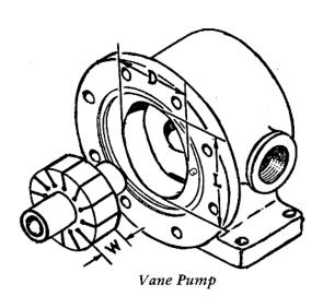
When replacing a pump, catalog ratings will usually be shown in GPM at a specified shaft speed. On motors, catalog ratings will usually be shown as C.I.R. (cubic inches displacement per shaft revolution). Formulae are shown for calculating either GPM at 1800 RPM or calculating C.I.R. Use the formula which is appropriate.
