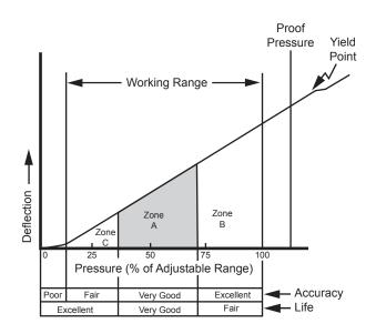
**Figure 1.** On switches with diaphragm and Bourdon tube movements, greatest accuracy is in the upper 65%, best life factor in the lower 65%, and the best combination is usually in the middle 30% of its working range (Zone A).
