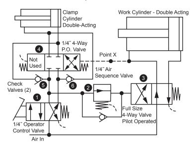
not available, a low range hydraulic relief valve can be used if it can be adjusted to about 50 PSI, and if the air line is lubricated. Refer to that sheet for more details.
