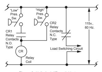
Figure 2. Unlimited differential between cut-out and cut-in pressures.
