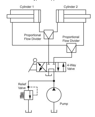
Figure 2. Flow dividers keep two unequally loaded cylinders moving at the same rate of speed, forward and reverse. Dividers split the flow equally to two cylinders of identical bore and stroke.
