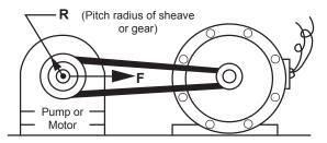
For pump:  $F = [HP \times 63,024] \div [RPM \times R]$ For hydraulic motor: F = T/R
