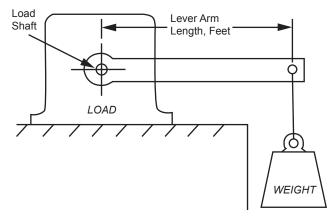
**Figure 1.** Breakaway torque of a load can be measured with a lever and weight, a spring scale, or a torque wrench.
