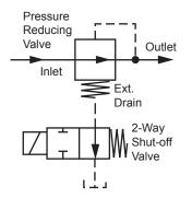
Figure 3. The 2-way valve shifts the outlet pressure from reduced setting to full system PSI.
