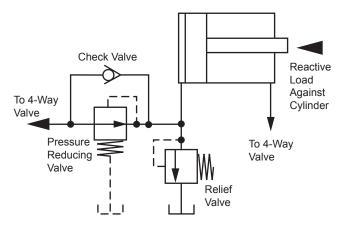
Figure 2. A highly reactive load may require the addition of a pressure relief valve on the reducing valve outlet.
