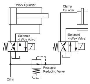
Figure 1. Reduced clamp pressure in a 2-branch circuit.
