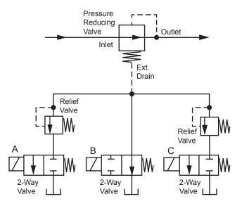
Figure 5. This circuit gives 4 pressure levels.
