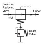
Figure 4. The relief valve allows a remote adjustment of the outlet pressure from reduced setting up to full inlet PSI.
