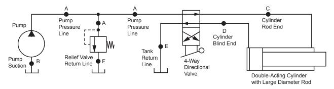
**Figure 1.** In different parts of the hydraulic circuit, flows and pressures are different. The optimum piping size for each line can be determined from permissible flow velocity and available pressure in each line
