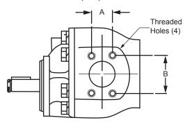
Figure 1. Many hydraulic components have 4-bolt port pads with standard SAE rectangular bolt spacing.
